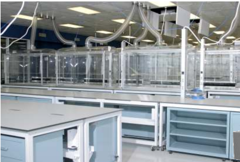
■ Above: Custom recirculating laminar flow cabinet with humidity control
